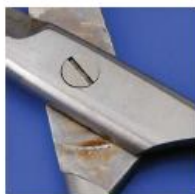
Example of Fretting Corrosion
